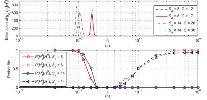
Fig. 5. The selection of threshold  $\varepsilon$  in Algorithm 1 given SNR = 15 dB,  $G_0 = 10$ , and  $P = 64$ : (a) estimated PDF of  $g_{\rho_1}(\rho_1|\mathcal{H}_1^0)$ ; and (b)  $\Pr(\mathcal{H}_1^1|\mathcal{H}_1^0)$  and  $\Pr(\mathcal{H}_1^0|\mathcal{H}_1^1)$  as the functions of  $\varepsilon$ .
