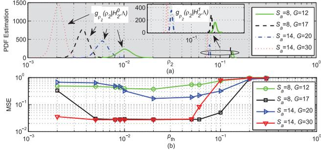
Fig. 4. The selection of threshold  $p_{th}$  in Algorithm 2 given SNR = 15 dB and  $P = 64$ : (a) estimated PDFs of  $g_{\rho_2}(\rho_2|\mathcal{H}_2^0, \Lambda)$  and  $g_{\rho_2}(\rho_2|\mathcal{H}_2^1, \Lambda)$ ; and (b) MSE performance of the DSAMP algorithm as the function of  $p_{th}$ .
