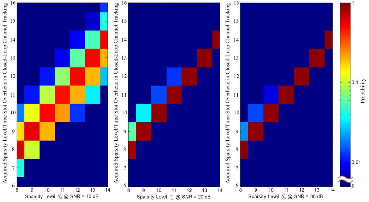
Fig. 10. Distributions of the acquired sparsity level  $\hat{S}_a$  by the CS based adaptive CSI acquisition scheme (which is then used as the time slot overhead for the proposed closed-loop channel tracking scheme) for different sparsity levels and SNRs.
