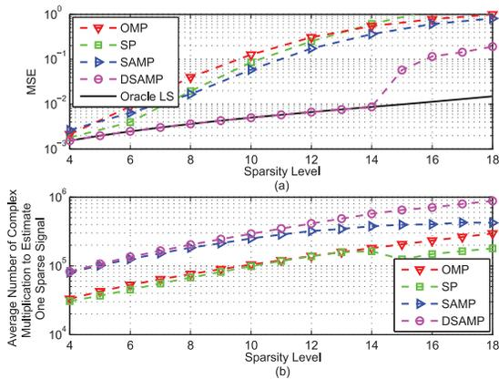
Fig. 6. Performance comparison of different CS algorithms as functions of the sparsity level  $S_a$  given  $G = 30$ ,  $P = 64$  and  $\text{SNR} = 20$  dB: (a) MSE performance, and (b) computational complexity.
