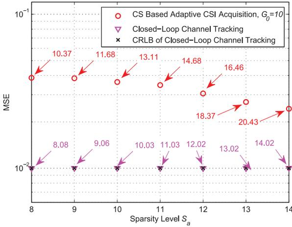
Fig. 11. MSE performance comparison of the CS based adaptive CSI acquisition stage and closed-loop channel tracking stage for different sparsity levels  $S_a$  at SNR = 20 dB, where the required  $\bar{G}$  for each case is indicated.
