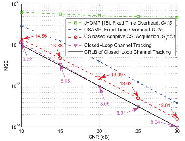
Fig. 12. MSE performance comparison of different channel estimation and feedback schemes for various SNRs and true sparsity level  $S_a = 8$ , where the required average time slot overhead  $\bar{G}$  for each case is indicated.
