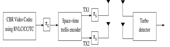
Figure 3: Schematic of the RVLC/CC/TC-coded and concatenated space-time trellis coded CBR video system employing turbo detection at the receiver. The notations  $\pi_c$  and  $\pi_s$  represent the channel interleaver and space-time trellis coding interleaver, respectively.
