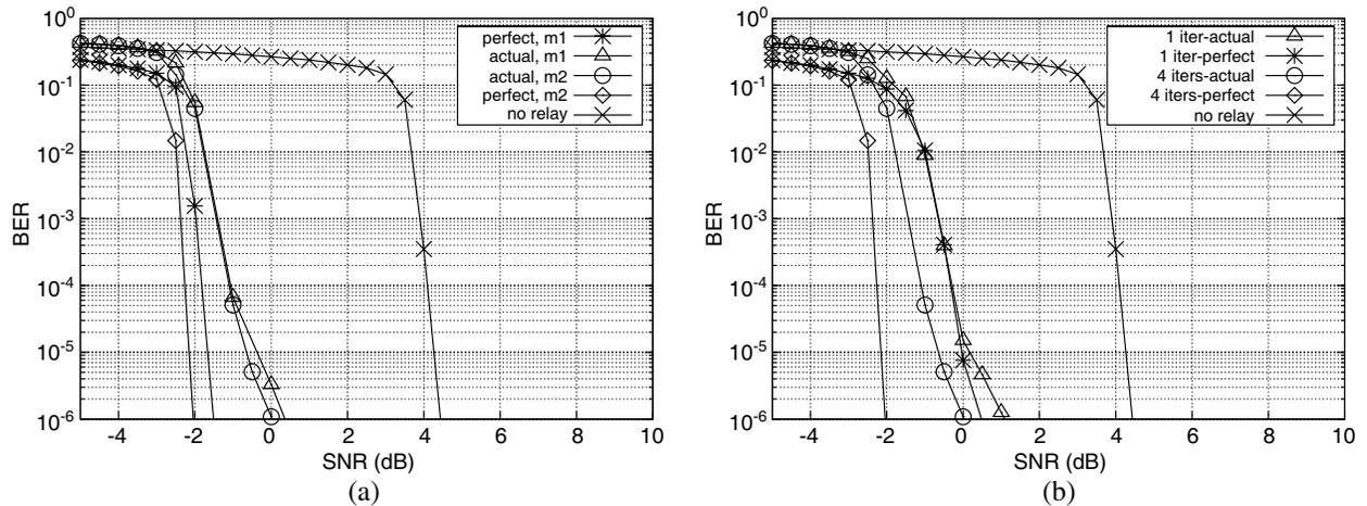
Figure 3: BER versus transmit SNR performance of the Turbo-coded CDMA-based two-way relaying system. MMSE detection is used in conjunction with  $P = 7$ -chip m-sequences in a  $K = 7$ -user CDMA system. A frame length of 12000 symbols is employed. (a) Performance comparison between the m1 and m2 models. (b) Effect of employing one and four Turbo decoding iterations.
