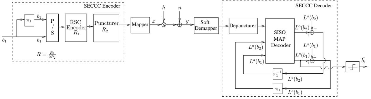
Fig. 3. Schematic of the SECCC encoder and decoder. The notation  $L(b)$  denotes the Log-Likelihood Ratio (LLR) of bit  $b$  and the superscripts  $a$ ,  $o$  and  $e$  denote the *a priori*, *a posteriori* and extrinsic nature of the LLR, respectively [15].
