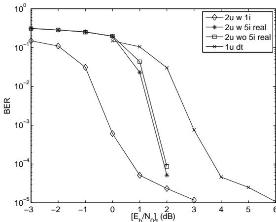
Fig. 6. BER versus  $[E_b/N_0]_t$  of Phase-II of the SPC-SECCC scheme for transmission over an uncorrelated Rayleigh fading channel.
