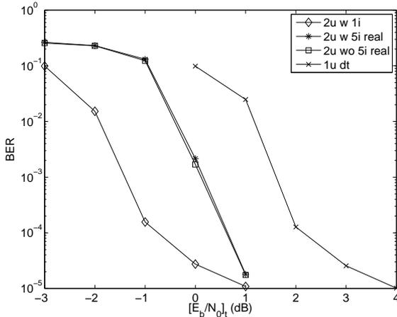
Fig. 5. BER versus  $[E_b/N_0]_t$  of Phase-II of the SPC-SECCC scheme for transmission over an AWGN channel.
