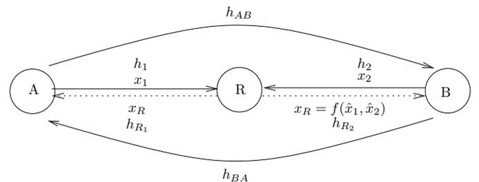
Fig. 1. Schematic of the bi-directional relay aided system.
