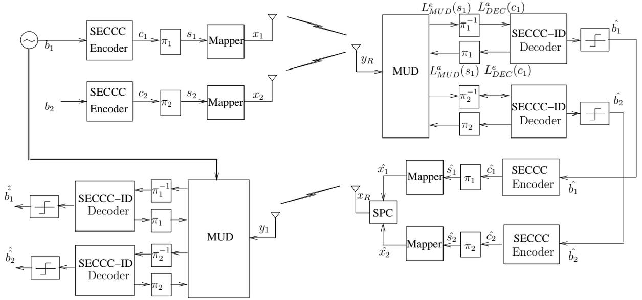
Fig. 2. SPC based SECCC-ID System (Phase I and II)
