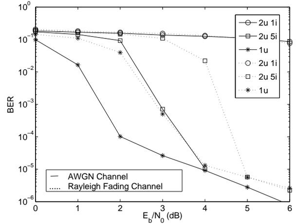
Fig. 4. BER versus  $E_b/N_0 = [E_b/N_0]_r$  of Phase-I of SPC-SECCC scheme for transmission over both AWGN and uncorrelated Rayleigh fading channels.
